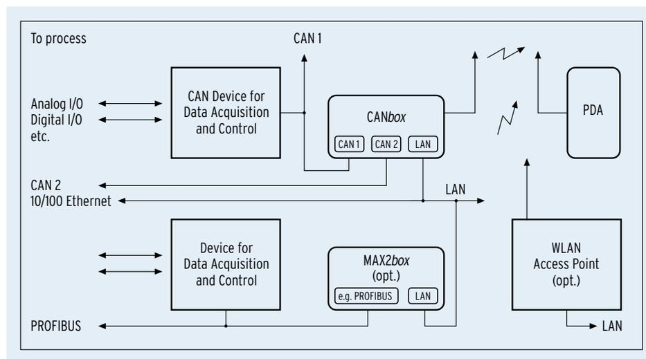
Example 2: Connection of 2 CAN buses via CANbox and WLAN to ARGUSpda. The Access Point and MAX2box are optional, e.g. for PROFIBUS.
