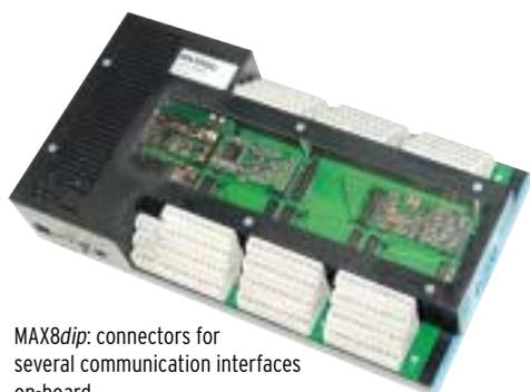
MAX8dip: connectors for several communication interfaces on-board
