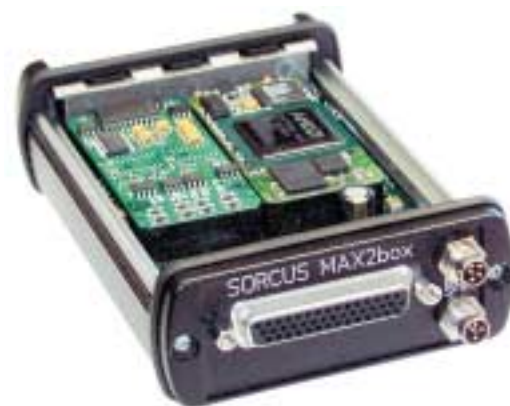
MAX2box: Stand-alone device for 2 resp. 3 MAX modules
